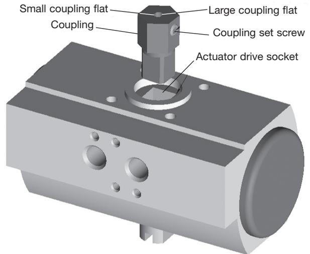
2. Place the **mounting bracket** on the **actuator** and orient in the desired position. Verify the **coupling** is in the proper position to maintain desired flow pattern.
