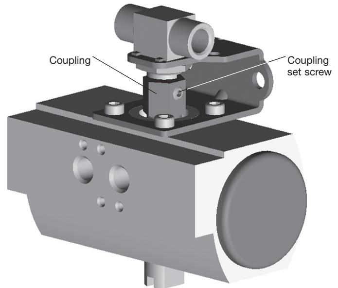
8. Test for proper valve operation by applying air pressure as specified by the actuator manufacturer.
