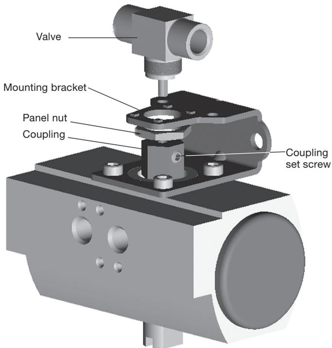
6. **40 series and SK series:** Position the **coupling** approximately 1 mm (0.04 in.) from valve body.
