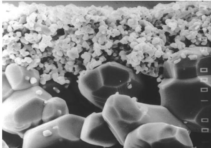
A scanning electron microscope image shows the two membrane layers of the filter: ultrafine and fine (as shown from top to bottom).
