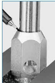
Swagelok depth marking tools help ensure that tubing is bottomed on the shoulder inside the Swagelok tube fitting body.
