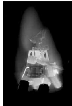
Actuator melted away.
