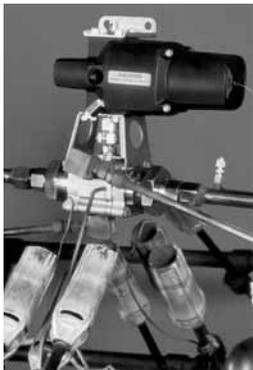
Pneumatically actuated fire series ball valve set up for burn.
