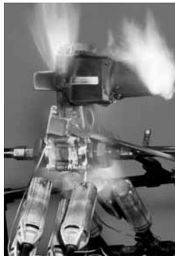
Actuator lubricants begin to burn off, and actuator begins to melt.
