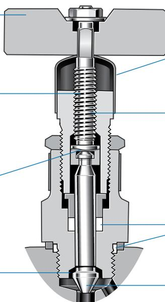
Shroud protects stem threads against ingress of dirt and dust
