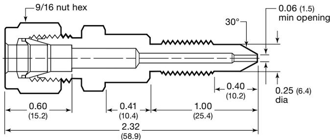
Calibration Fitting with 1/4-28 in. Thread
