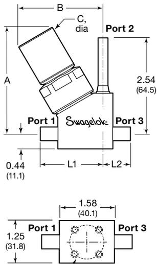
Four mounting holes, M5 × 0.8-6H thread, 0.25 (6.4) deep, 45° from center line, on a 1.00 (25.4) bolt circle. M5 × 0.8-6H holes are compatible with 10-32 mounting screws.
