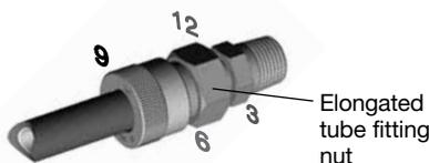
7. While holding the fitting body steady, tighten the elongated tube fitting nut one and one-quarter turns to the 9 o'clock position.
