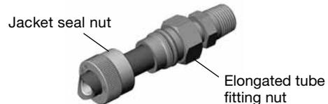
2. Tighten the jacket seal nut hand-tight. The jacket seal nut will cover the vent O-ring when it is sufficiently tightened. If desired, perform a *pressure decay* leak test.
