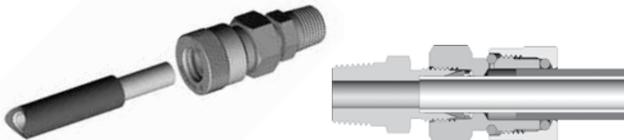
6. Mark the elongated tube fitting nut at the 6 o'clock position.
