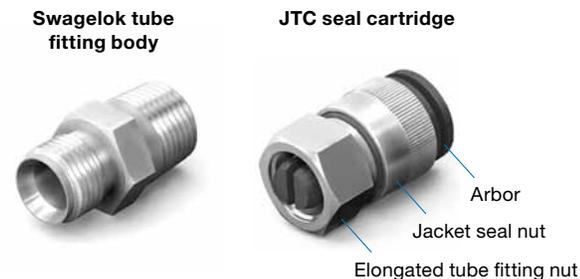
The preassembled JTC seal cartridge assures installers of the correct ferrule orientation and proper installation into the fitting body. Components are released only after the tube fitting nut is threaded finger-tight onto the tube fitting body.
