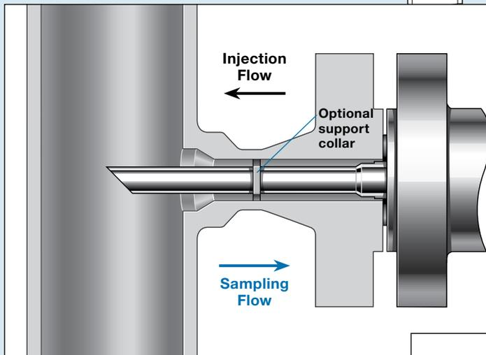
**Injection Valve Flow Compared with Sampling Valve Flow**
