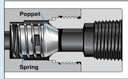
**Injection Valve with Integral Check Valve and NPT Connection**
