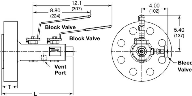
**Raised-Face (RF) Flange Process and Outlet Connections**
