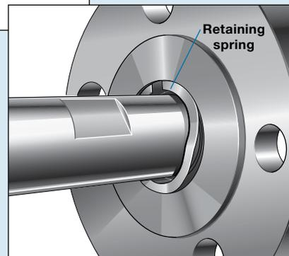
A process interface valve fitted with an injection probe and a check valve allows fluids to be dispersed into the process stream while providing protection against back flow of process fluids.
