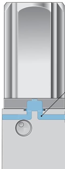
Flow path to the analyzer is fully swept, enhancing the rate of system purging.
