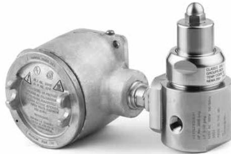
The KEV series is an electrically heated vaporizing regulator with a low internal volume. It can be used to vaporize liquid samples or to preheat gas samples to prevent them from condensing. It features a heating element that is in direct contact with the process fluid for maximum thermal efficiency and is removable for easy cleaning. The KEV regulator has an integral temperature controller and is rated for use in hazardous areas, as identified below.
