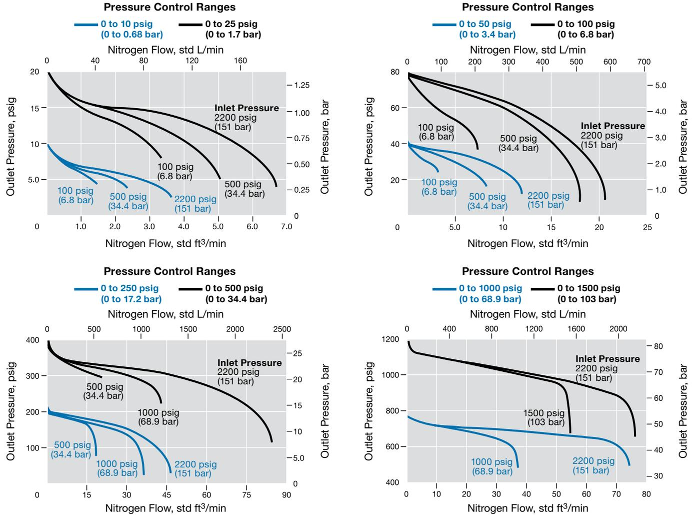
**Flow Coefficient 0.20; Maximum Inlet Pressure 3600 psig (248 bar)**
