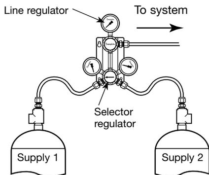
The selector regulator (first stage) is factory-set to reduce the supply pressure to the nominal changeover pressure ordered. The line regulator (second stage) can be adjusted with the handle to achieve the required system pressure. This two-stage arrangement minimizes the supply-pressure effect caused by depleting gas supplies (cylinders, tank farm, etc.).
