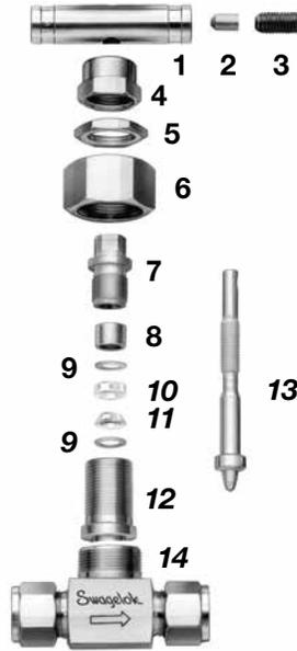
**⚠ To increase service life, ensure proper valve performance, and prevent leakage, apply only as much torque as is required to achieve positive shutoff.**
