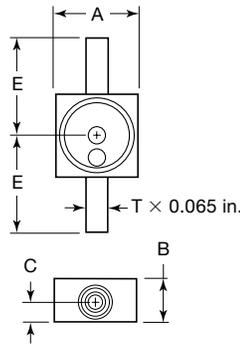
Shown with TB (tube butt weld) ends
