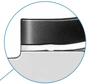
Flexing at the point of seal during cycling
