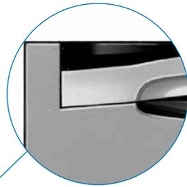
No flexing at the point of seal sustains the seal integrity during cycling
