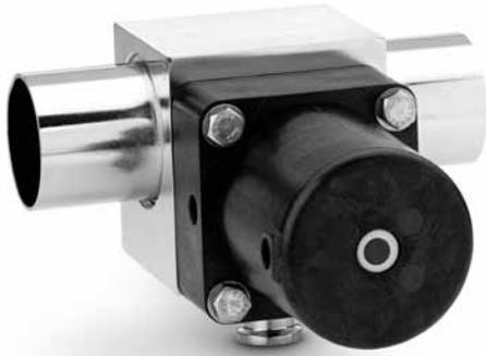
**Point-of-use valve with plastic pneumatic actuator, straight tube extension header, and TS series sanitary clamp fitting at takeoff port**
