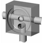
Typical 1-valve configuration with 3 ports
