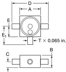
Shown with TB (tube butt weld) ends
