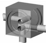
Typical 2-valve configuration with 3 ports
