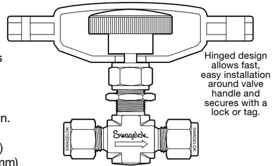
Hinged design allows fast, easy installation around valve handle and secures with a lock or tag.
