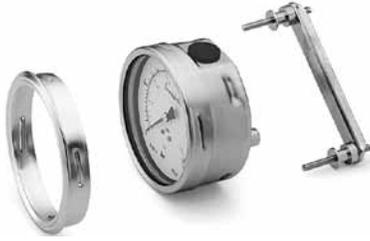
Stainless steel panel-mount clamps are available for flush mounting Swagelok industrial gauges. The panel-mount clamp is easily installed on the gauge. This option is not available on lower mount or S model gauges. Panel-mount clamps on M model gauges must be factory installed and are available as accessories for field installation on B, C, L, and P model gauges.
