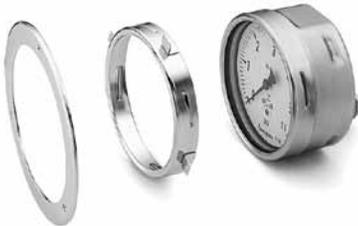
Polished stainless steel front flanges are available for flush panel mounting of Swagelok industrial gauges. This option is not available on lower mount or P model gauges and must be factory installed on C and M model gauges.
