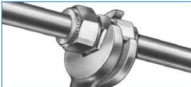
1. Install the Swagelok nut and ferrules onto the preswaging tool.
