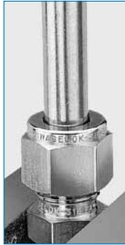
1. Insert cleanly cut, fully deburred tube into the depth marking tool (DMT) until the tube is against the shoulder of the tool. Using a pen or pencil, mark the tube at the top of the DMT (Fig. 1).
