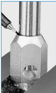
Swagelok depth marking tools help ensure that tubing is bottomed on the shoulder inside the Swagelok tube fitting body.
