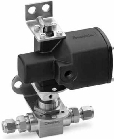
Swagelok rack and pinion pneumatic actuators are compact, lightweight, easily mountable, and can be operated with standard shop air. They are available in spring-return and double-acting modes. On-off (2-way) valves require 90° actuation; switching (3-way) valves require 180° actuation.
