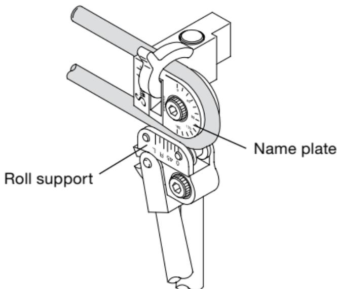
6. After completing the bend, swing the **short handle** away, pausing when the 0 on the **roll support** reaches approximately 90°. Loosen the short handle, move it until parallel with the long handle, then retighten the short handle.
