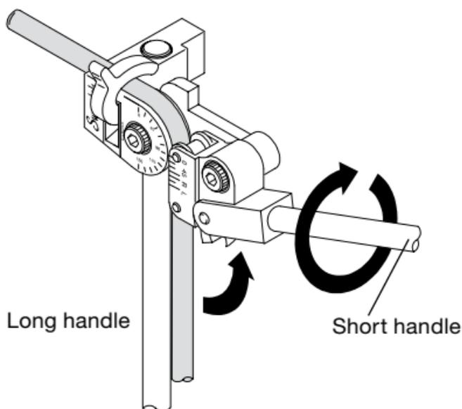
5. Continue the bend until the 0 on the **roll support** reaches the desired degree mark on the **name plate**.
