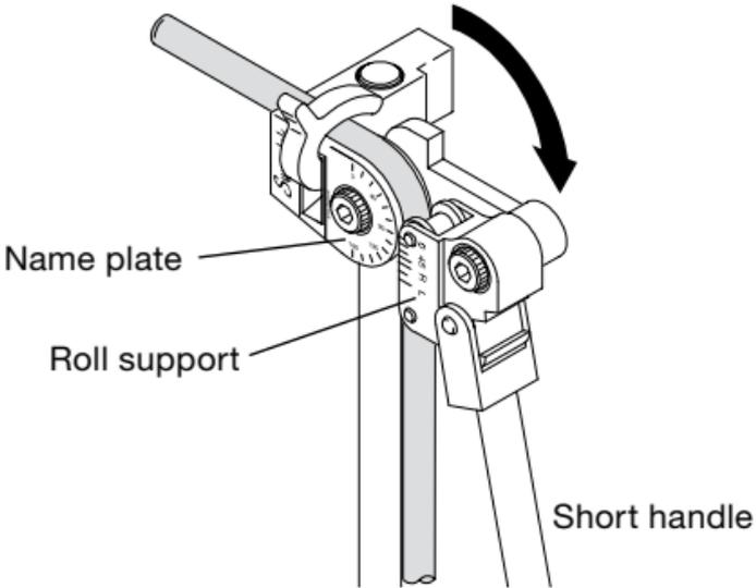
2. Loosen the **short handle** from the **clevis** until the short handle will swing without moving the **roll support**.
