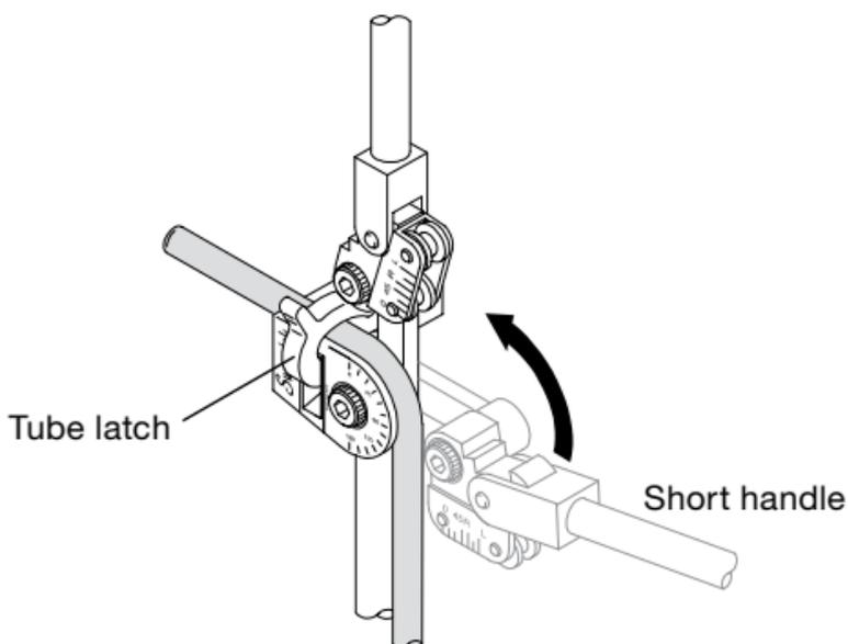
3. Pull the **tube latch** off the tube and remove the tube from the bender groove.
