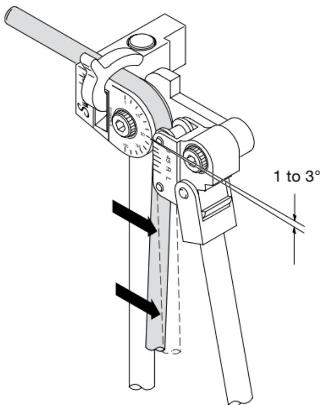
Note: Do not bend all the way to the bend mark when bending softer tubing such as copper or aluminum.
