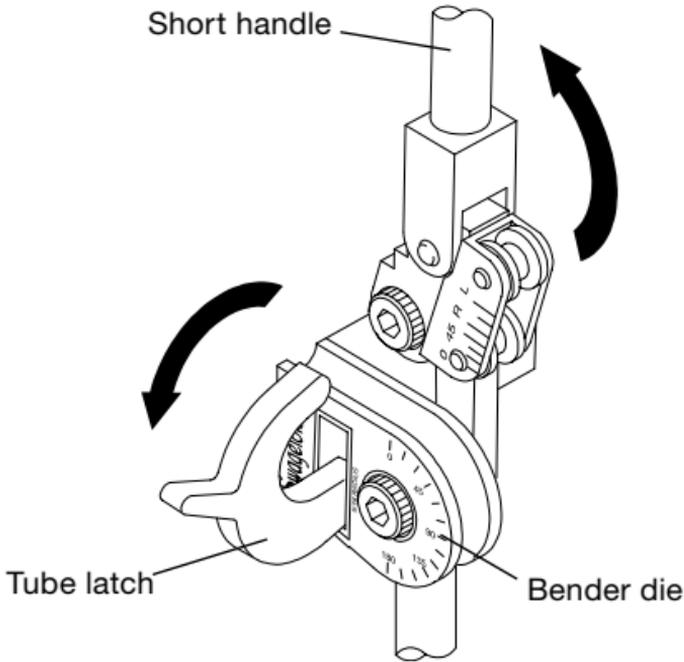
3. Place the tube in the groove of the **bender die** with the **reference mark** to the left of the **tube latch**.
