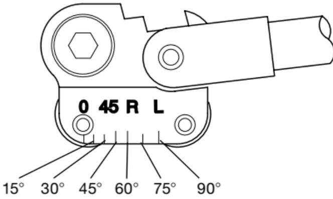
Note: View the marks on the hand tube bender as a 0 to 90° scale when bending other angles.
