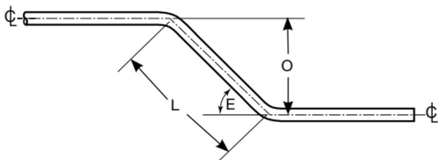
The purpose of an offset bend is to change the center line of the run, typically to avoid an obstruction. To determine the length of offset, select the offset angle (E). Then, multiply the offset dimension (O) by the offset bend allowance (A).
