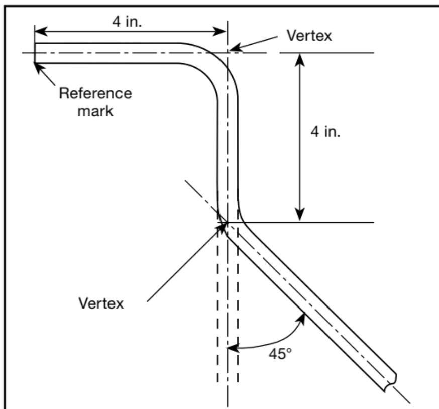
1. Place a **reference mark** at the end of the tube from which you are beginning the measurements.
