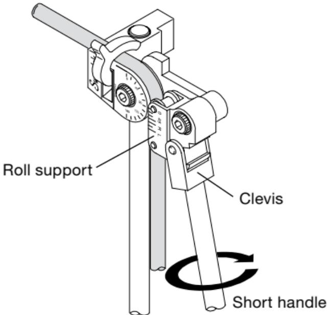
3. Swing the **short handle** up until it is slightly above perpendicular to the **long handle**.
