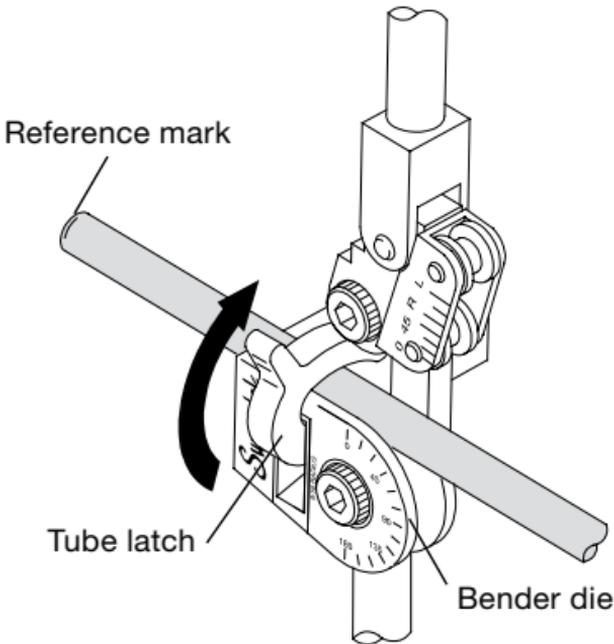
5. Carefully lower the **short handle** until the **roll dies** rest gently on the tube while keeping the **link** straight and parallel to the **long handle**.
