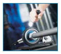
Preswage the Swagelok nut and ferrules onto the tube using the multihead hydraulic swaging unit;
