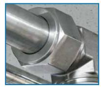
align and insert the tube into the Swagelok fitting;
