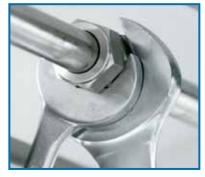
turn the nut hand-tight, then tighten one half turn with a wrench.
